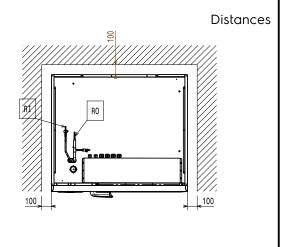
**Electric** Circuit breaker required Supply voltage: 380-415 V/3N ph/50/60 Hz Heating power: 6.4 kW Water: Drain line size: Pressure, bar min: 0
